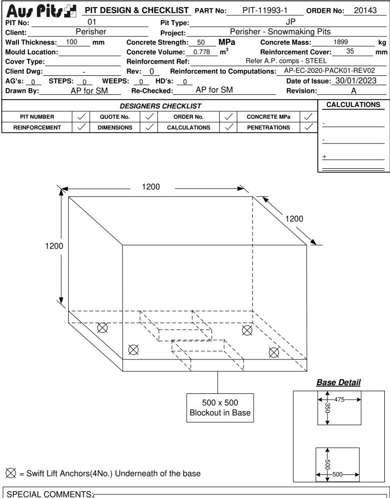
Lifting anchors will be on the underneath of the base
